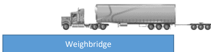
Figure 12: Semitrailer and dolly weighed with dolly off the weighbridge
