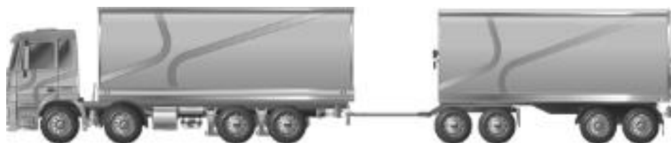
Figure 40: Example twin steer truck (Code 73 – 4 Axle Twin Steer Rigid Truck & 4 Axle Dog Trailer)
