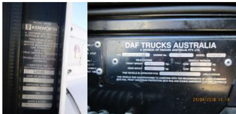
Figure 11: FUPs bar compliance plates
